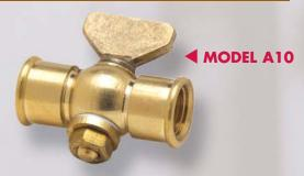
In polished brass (suitable for pressure to 125 PSI hydraulic) Specify Type A10 1/4" NPT female connections. A11 1/4" NPT male x female
