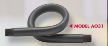
Schedule 40 Steel (for max. 500 PSI and 400°F) Specify Type **A03I**. 1/4" NPT. Brass (for max. 250 PSI and 400°F specify type **AO3B**.
